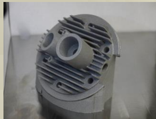
UAV engine component produced using 3D metal printing technology under a NAVSEA STTR with WIU and IDRC
