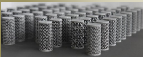
Titanium Lattice Structures Produced by 3D Metal Printing
