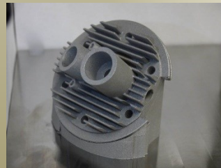
UAV engine component produced using 3D metal printing technology under a NAVAIR STTR with WIU and IDRC
