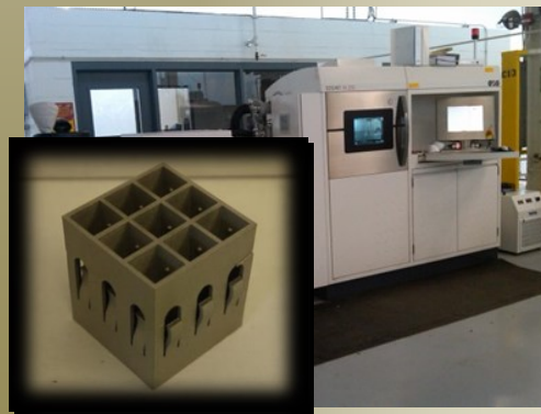
Powder Bed Fusion 3D Metal Printing System and Component Fabricated by 3D Metal Printing
